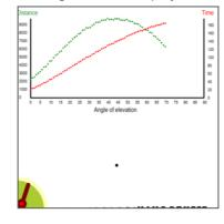
gram shown here (with smashed balls littering the ground and one in flight), gradually raises the cannon from 0° towards 90°, building up graphs to show how flight time and distance vary with the initial angle. Students thus gain a deeper, practical appreciation of the relevant theory, from the trigonometric calculation of initial x and y velocities, to the application of gravitational acceleration to the *y* velocity.
